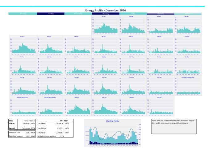
There is a peak around 8am in the morning, which is to be expected, as the main daytime systems start to run. There is then a relatively consistent load through the rest of the day. There is some correlation to the weather (outside air temperature) but it is not well aligned. This would seem to suggest that there are systems remaining on constantly regardless of occupation or weather and further sub metering of the main blocks would be required to analyse the usage further.
